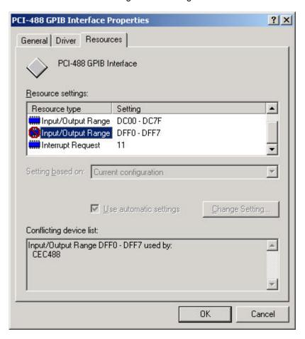
If the View menu is used to select "resources by connection", then an hierarchical view is presented. This again shows "CEC488" using the same I/O range as the "PCI-488 GPIB Interface".
